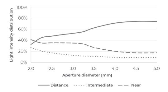
The light intensity measurements support the MTF simulation: as the aperture changes, the light distribution among the focal points changes accordingly.
